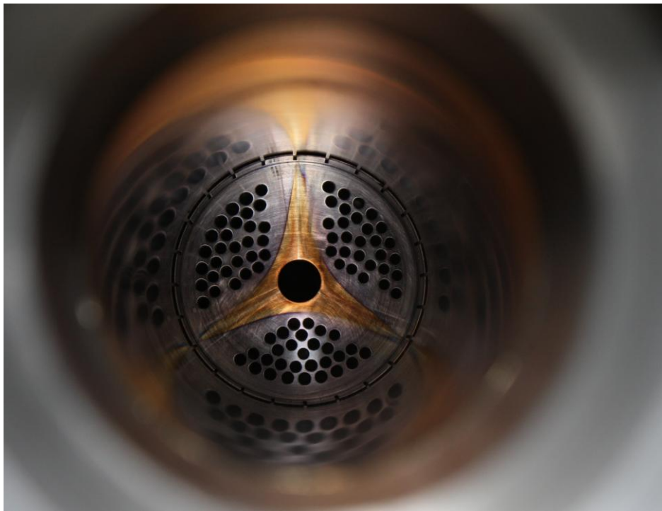
Figure 4. The yellow triangle on the extraction electrode shows the lost gold particles.
