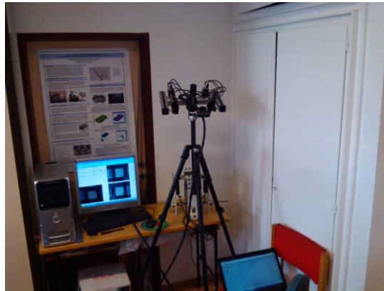
Figure 5: VIALUX system & bi-axial stress measuring
