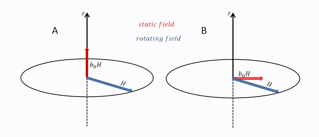
Two cases are considered: (T = 0)A)  $b_0 \perp$  rotating field ? rotating field  $(b_0 = 0)$ B)  $b_0 \parallel$  rotating field ? rotating field  $(b_0 = 0)$
